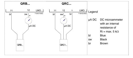
As an alternative to detector current measurement, the diagnostic tool OCI400 / ACS400 / ACS410 can be used. In that case, connection of the DC microammeter is not required.
