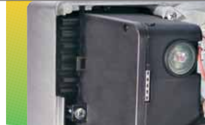
Control-box fitted with ignition transformer
